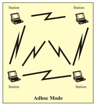
In infrastructure mode, all stations in a system connect to an Access Point and not directly to one another. In adhoc mode, the stations interconnect directly, without communicating through an Access Point.
